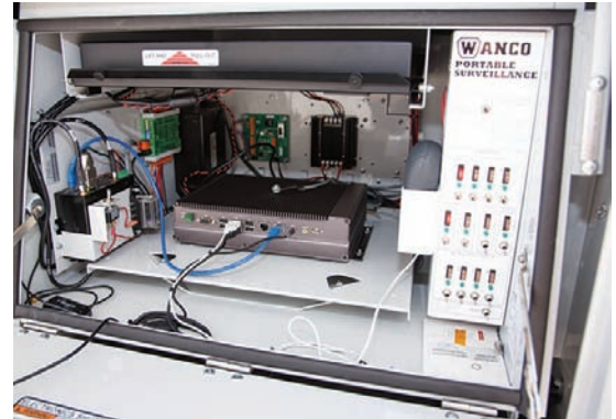
Equipment bay houses electronics, including DVR, monitor and communications
