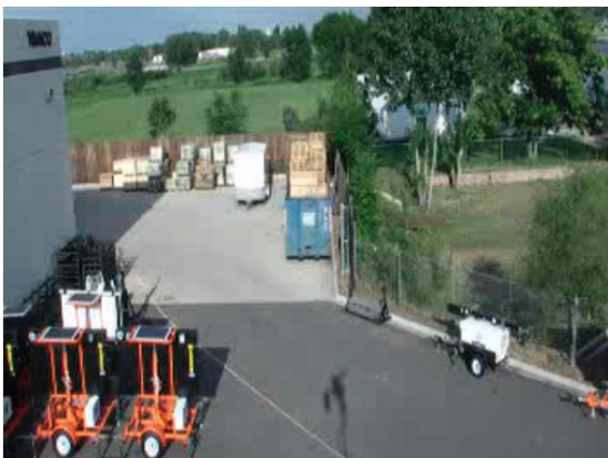
Streaming video (during remote viewing) can be compressed, with reduced resolution and lower frame rate, to conserve cellular bandwidth
