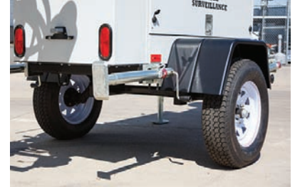
Off-road package adds wider axle and heavy-duty drawbar wheel
