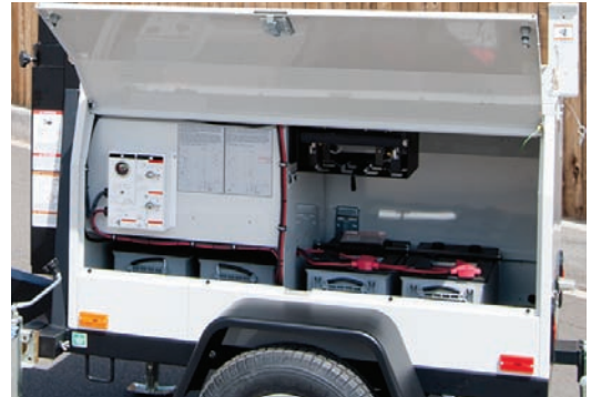
Batteries located inside locking equipment cabinet, separated from electronics
