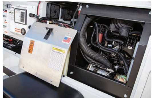
Diesel engine in self-contained compartment with removable cover
